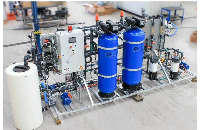
Skid mounted BWRO & MMF plant
