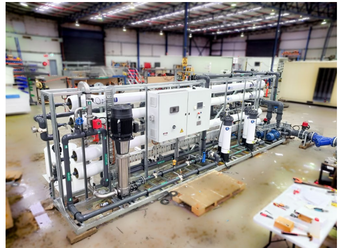
BWRO in construction at Perth factory
