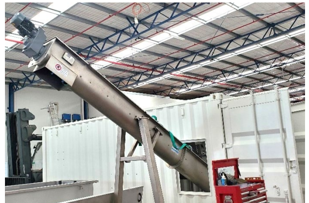
Containerised DSP and Screw Conveyor plant under construction in MAK Water factory
