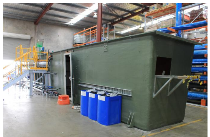
Modular design FRP bioreactor in Perth Fabrication facility
