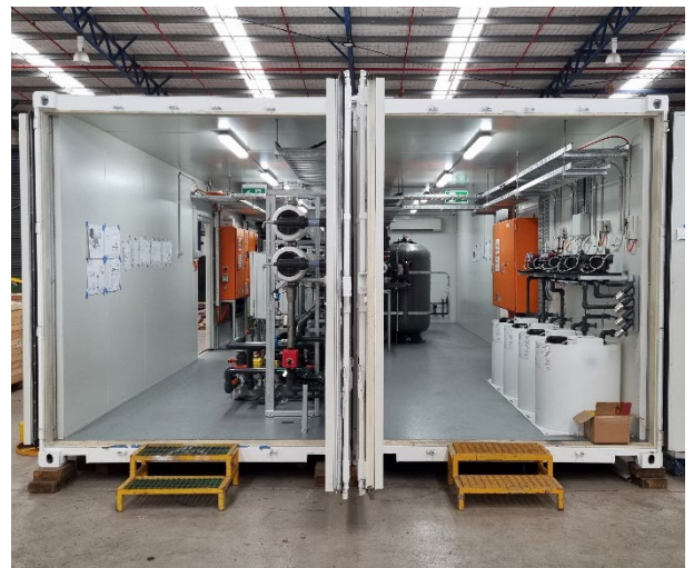
RO + CEDI and MMF + Chemical dosing containers side-by-side in factory
