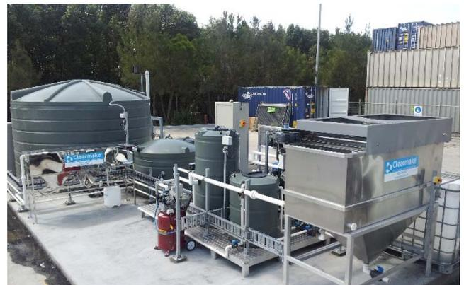
*The system uses hydroxide precipitation, flocculation and DAF clarification to remove silt, heavy metals, seeds, weeds and pests from the water*
