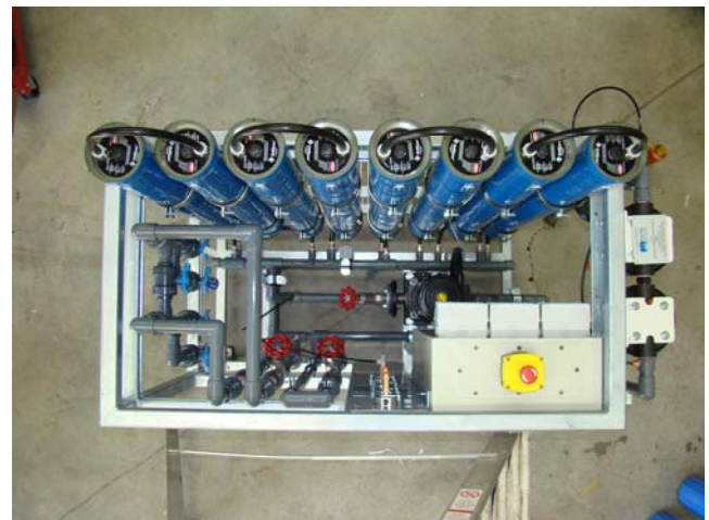
Demineralised Water Reverse Osmosis Plant
