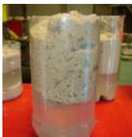
DAF SLUDGE: - Looser Flocs - Tend to Sink - Not Immediately Decantable
