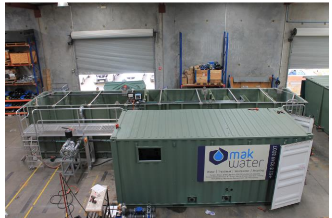
MBBR plant in MAK Water's workshop
