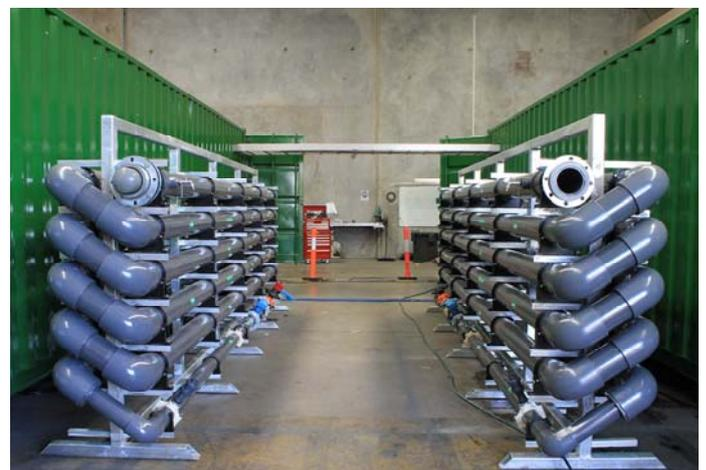
*Two off skid mounted tube flocculators and containerised multimedia filtration plants*
