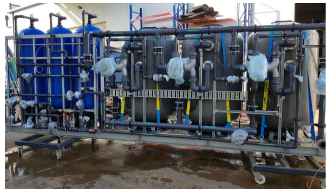
Custom design and manufacture of a skid mounted Multimedia Filtration Plant for PFAS removal
