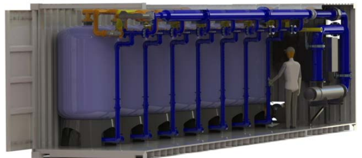
3D model MAK Water MMF plant
