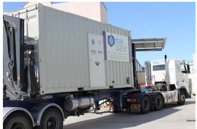
330 m 3 /day containerised MMF plant loaded for transport to Kazakhstan
