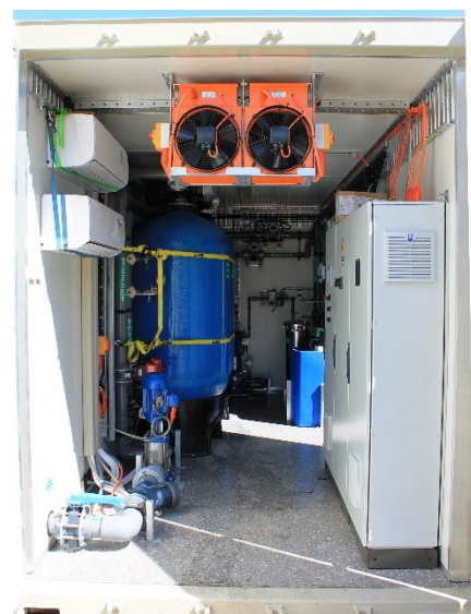
330 m 3 /day containerised MMF plant ready for delivery to site
