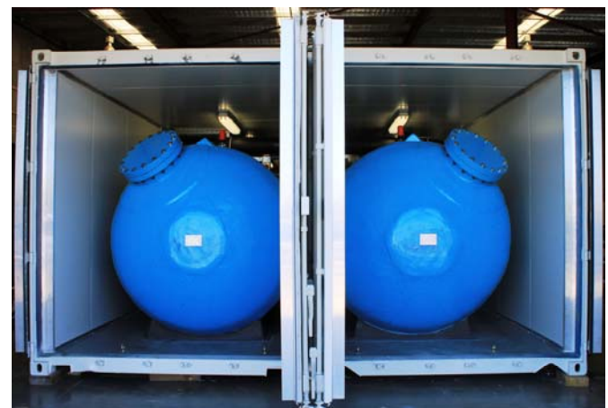
MMF plant undergoes Factory Acceptance Testing in MAK Water's workshop
