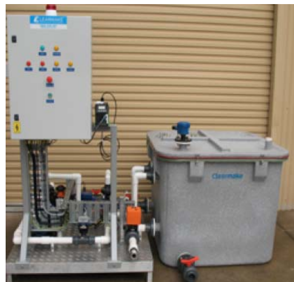
pH Adjustment Plant
