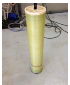
Membranes at the same age, using the MAK Water S5 antiscalant resulting in a longer membrane life and lower dose rates required
