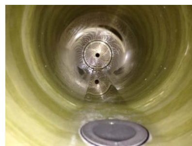
Membranes at the same age, using the MAK Water S5 antiscalant resulting in a longer membrane life and lower dose rates required
