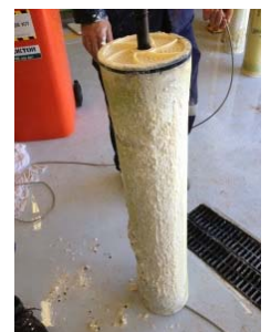
Membranes using an inappropriate antiscalant resulting in degradation of the membranes and subsequent shorter lifespan
