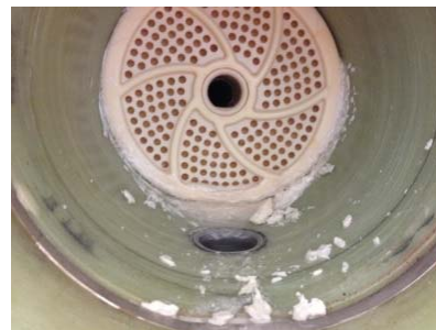
Membranes using an inappropriate antiscalant resulting in degradation of the membranes and subsequent shorter lifespan
