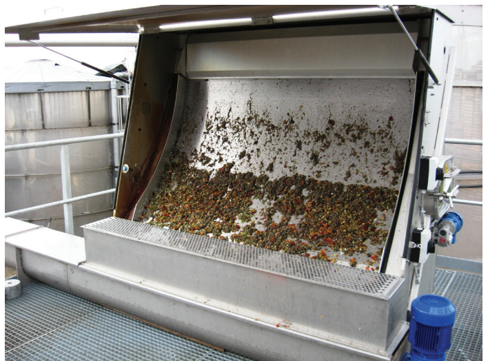
Typical Reko Static Bow Screen with optional Hinged Cover, Integrated Automatic Cleaning System and Screw Conveyor
