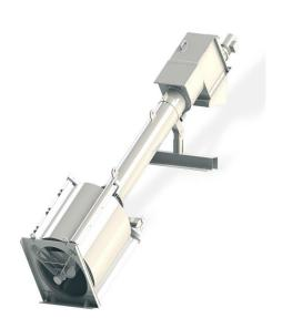
The floating and suspended materials (screenings) in the sewage enters in the basket and forms a mat on the screen element which increases the level upstream of the screen. A level sensor sends a signal to start the rotation of the screw screen and the outer rotary loading drum.
