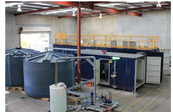
MAK Containerised MBBR undergoes FAT in MAK's Workshop
