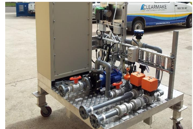
MAK skid mounted pH Adjustment plant
