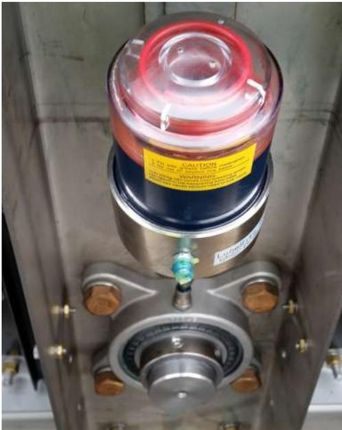
Figure 6. Typical automatic Lubesite lubricator on non-drive end bearing & shaft (housing cover removed for clarity)
