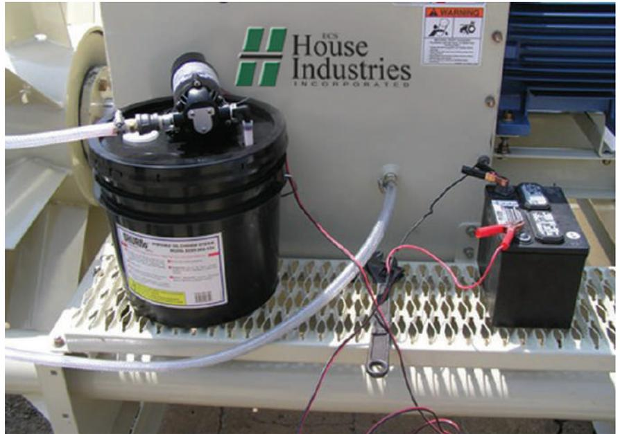
Figure 7. Gear Reducer oil change being completed using oil change kit supplied with Floating Brush Aerators
