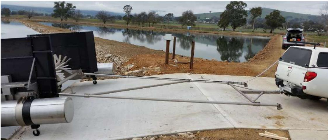
Figure 5. Corryong WWTP Floating Brush Aerator with special rolling assembly
