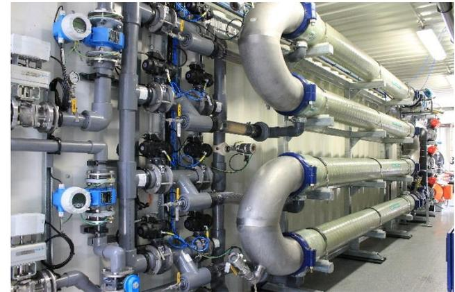
Containerised UF & Chemical Dosing Systems, with
