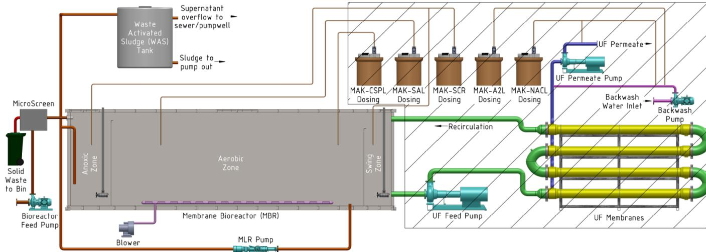
The MBR process is a suspended growth activated sludge system that utilises microporous membranes for solid/liquid separation in lieu of secondary clarifiers.
