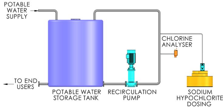
In order to treat the raw water to Australian Drinking Water Guidelines (ADWG) sterilisation is required. Free chlorine residual in the potable water storage tank is automatically maintained by providing a recirculation system with sodium hypochlorite dosing.
