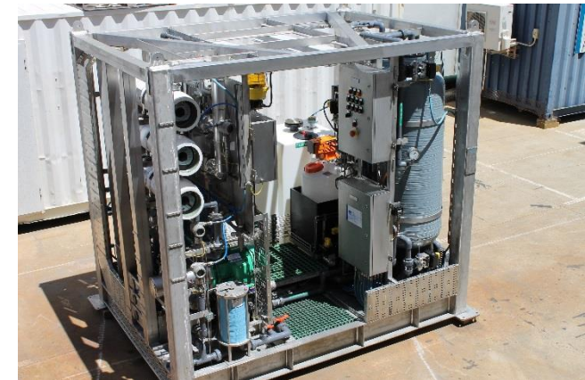
MAK Skid Mounted 40 m³/day SWRO Plant for Offshore Oil Platform (Zone 2 Hazardous Area)
