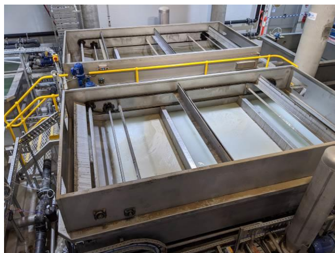
DAF pre-treatment to remove TSS and Oil & Grease
