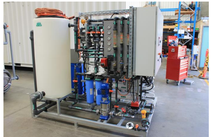
Skid mounted BWRO plant prior to despatch
