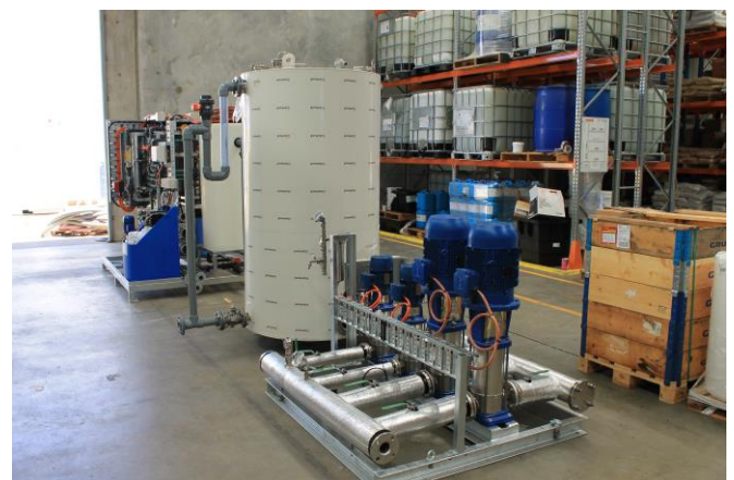
Recirculation and distribution pump skid with SS tank
