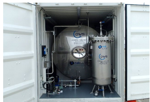
9,240 litre 316 stainless steel storage tank
