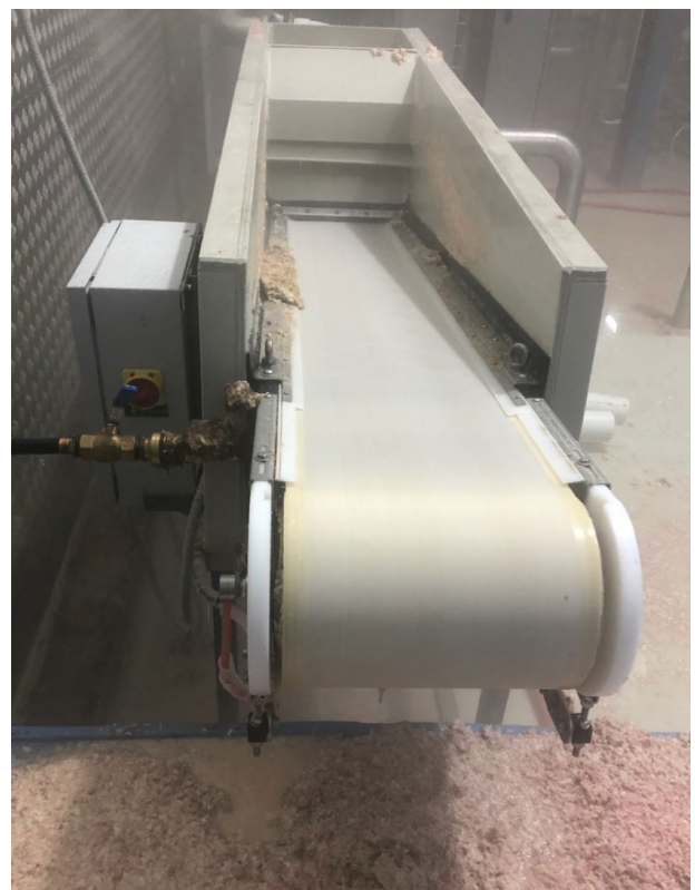
Belt Filter Trial on Site
