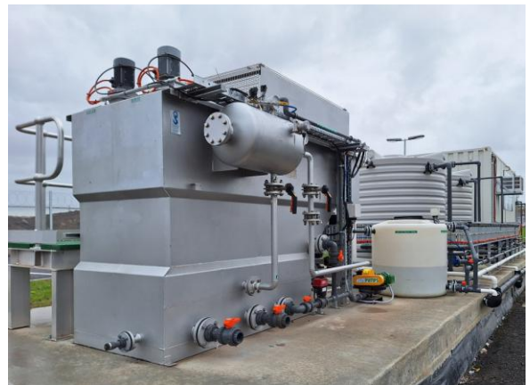
Dissolved Air Flotation (DAF)
