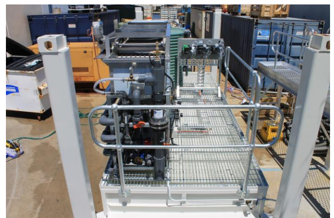
Side view of MAK Water Oil Water Separator
