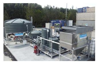
The system uses hydroxide precipitation, flocculation and DAF clarification to remove silt, heavy metals, seeds, weeds and pests from the water
