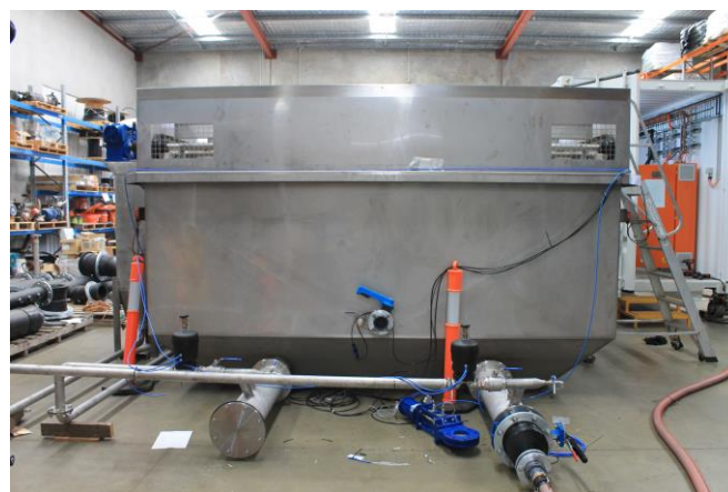
4,800 m 3 /day Dissolved Air Flotation (DAF) plant
