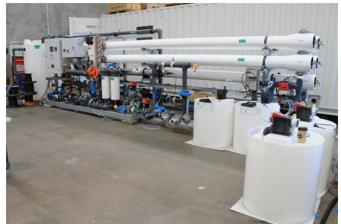
Skid mounted DWRO in Perth fabrication facility during Factory Acceptance Testing (FAT)
