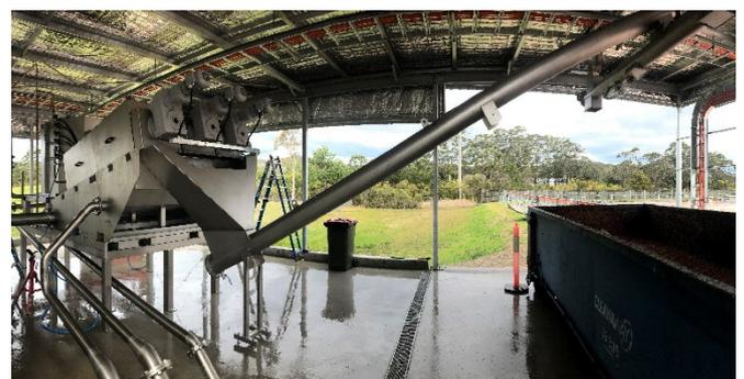
*Dewatering Screw Press DSP-403 with automated screw conveyor and outloading system.*
