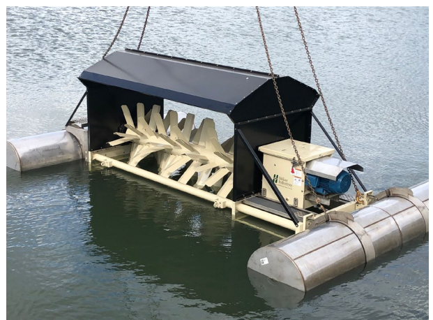
Floating Brush Aerator with rotor covers removed during installation
