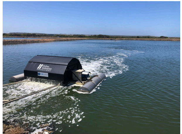
Typical Aeration & Mixing pattern by Floating Brush Aerators
