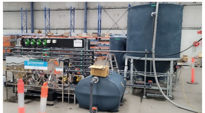
Oil-Water Separator; Gravity Clarifier; Chemical Dosing Pumps and ancillaries in the MAK Water factory
