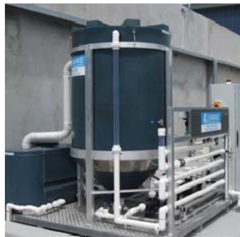
The Gravity Clarifier system is capable of treating 1,500 litres per hour of wash water.
