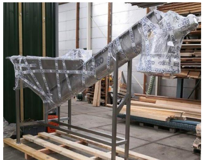
Screw separator / grit classifier packaged and ready for delivery
