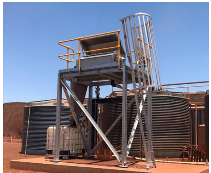
Internal Fed Drum Screen Installed and in operation.
