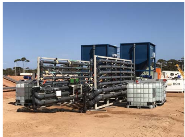
Custom RO Pre-Treatment plant installed onsite
