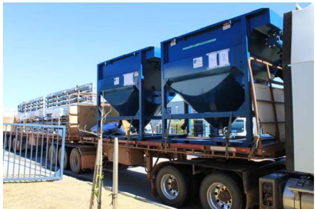
Lamella Clarifiers with flocculation and dosing skids
