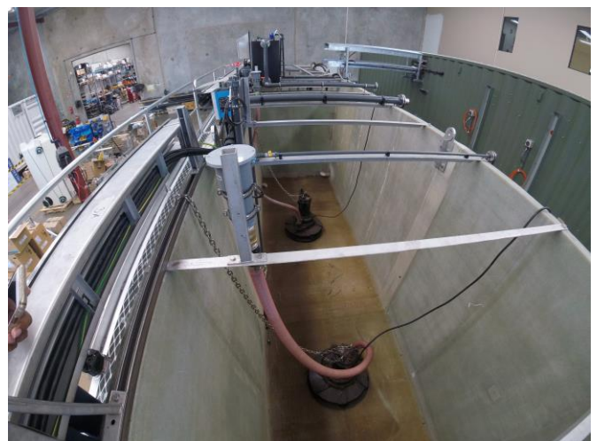
Corrosion resistant fibre-reinforced plastic (FRP) bioreactor
