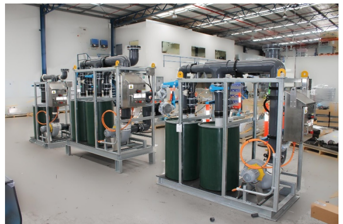
Carbon odour filters treat plant biogas emissions
