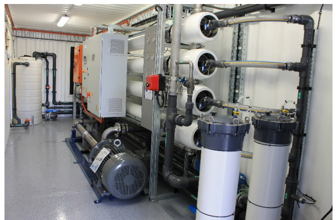
Containerised SWRO plant undergoes factory acceptance testing
