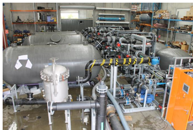
4,800 m 3 /day skid mounted Multimedia Filtration (MMF) plant
