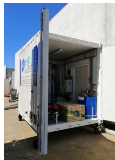
Compact containerised (1 x 10') with air conditioning and non-slip floor coatings
