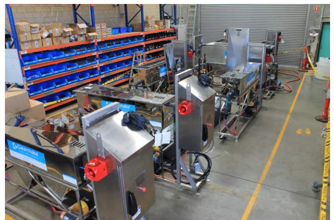
8 x Clearmake™ OWS in the Perth Fabrication Facility prior to dispatch
