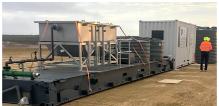
Skid-mounted OWS and containerised delivered to site
