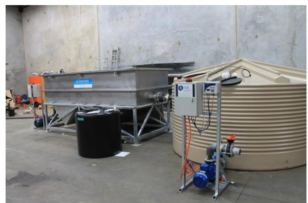
Package was supplied with a treated water tank and transfer pump
