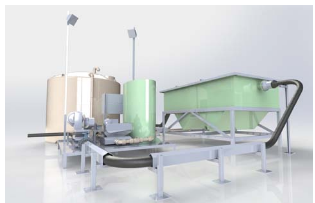
3D drawing of the MAK Water Oil Water Separator installed on-site
