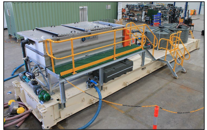
MAK Water OWS system installed on a 40' flat rack
